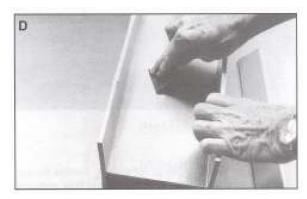
4. Many users paint the Exel Composites structural shapes to enhance surface appearance. Structurally, the synthetic veil enables Exel Composites FRP to suffer only minimal damage due to ultraviolet radiation; however, some fading of the surface pigmentation will be observed. This surface fading can be minimized by painting.
