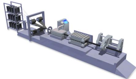
In pultrusion process the fibers are impregnated with a thermoset resin and pulled through a heated die where curing takes place.
